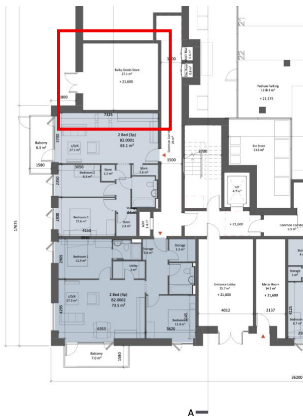
Figure 8: Extract from Architectural drawing showing typical location of bulky storage in Apartment Block 1 (highlighted in red)
