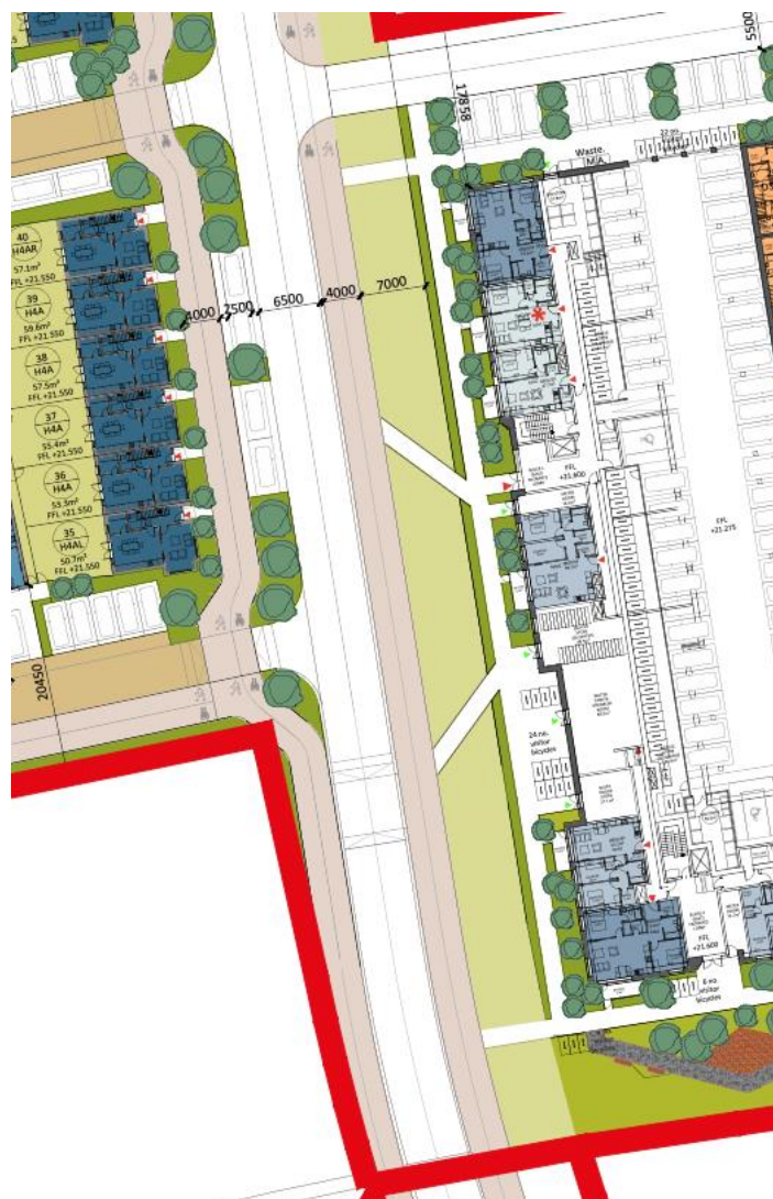
Figure 6: Extract from Proposed Site Layout drawing 24004-OMP-00-SP-DR-A-1000 showing the relationship and interactions between Blocks 1/2 and LUAS reservation corridor prepared by O'Mahony Pike Architects.
