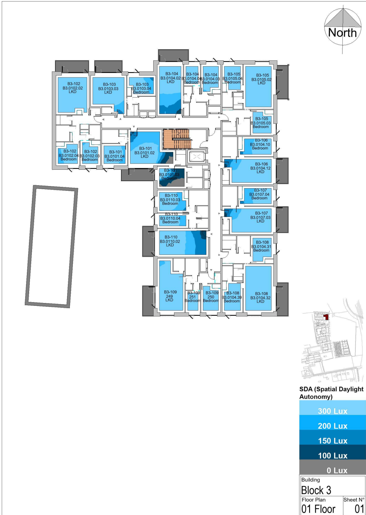
Figure 13 Block 3 Floor Plans with Daylight Heatmaps
